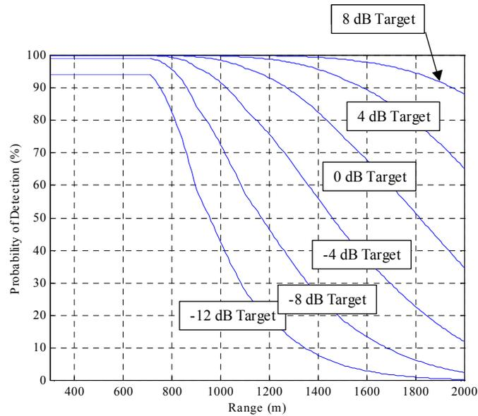
**Figure AA-10. Probability of detecting objects of various TS assuming object resides at midpoint of mainlobe (9 dB per km absorption).**
