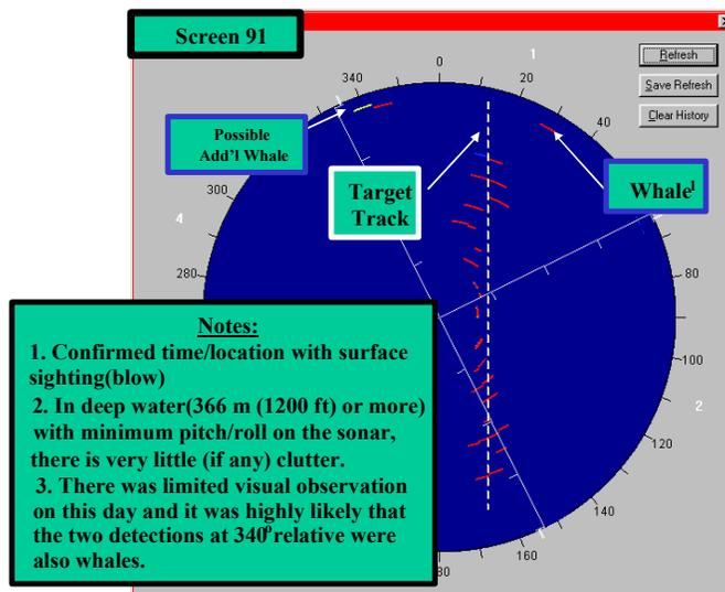
Figure B-10. Detection/Tracking Screen Showing Target (-2 dB) and Whale Detections.
