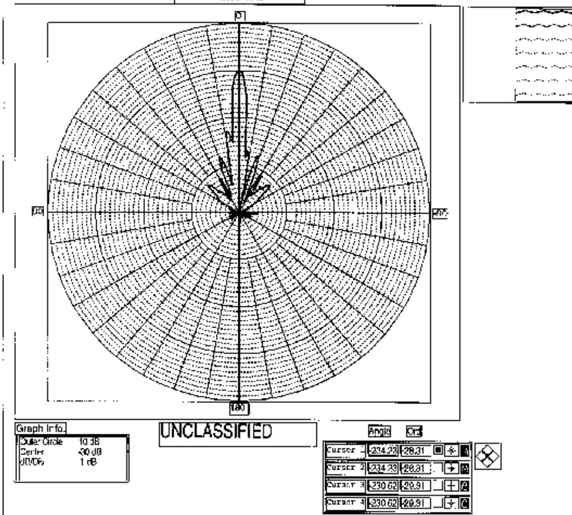
Figure B-19. Nominal Measured Transmit Beam Pattern for Parabolic Reflector at 40 kHz.
