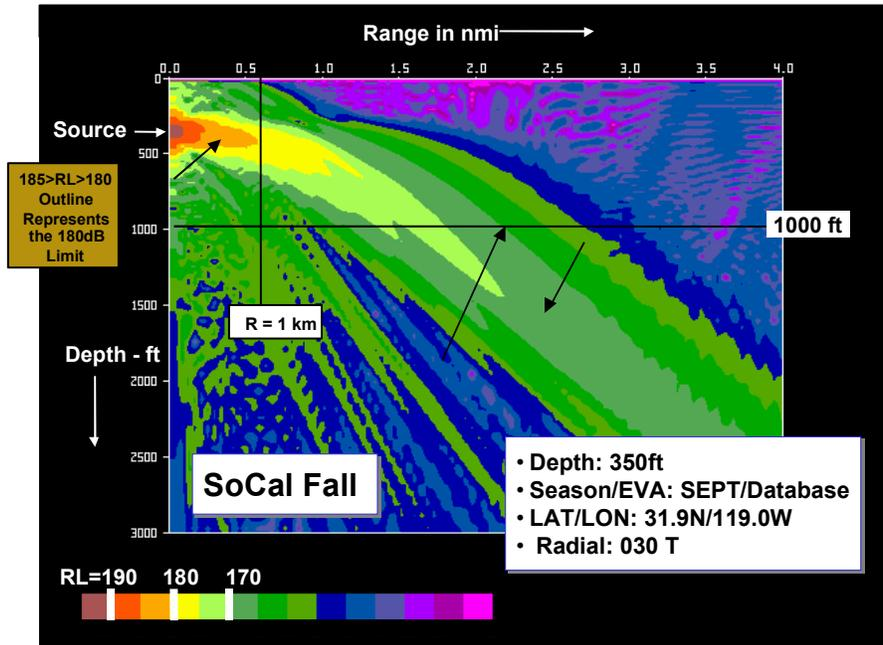
Figure A-3. PE Run for the LFA Array.
