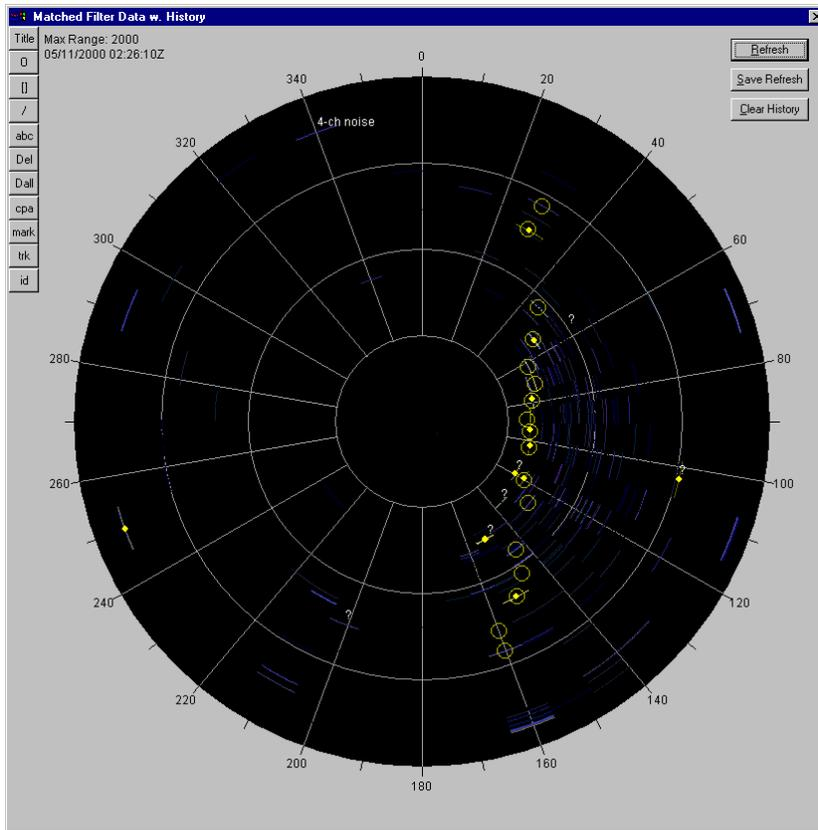
Figure 4. Polar display of HF/M3. The figure displays multiple detections of a small, artificial target drifting past the HF/M3 sonar.
