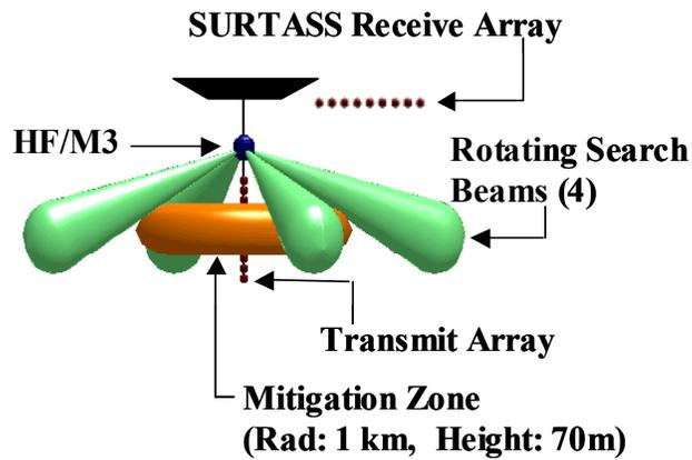
Figure 2. System concept schematic.
