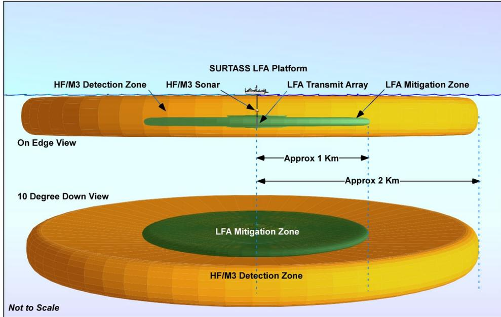
Figure A-1. HF/M3 Sonar Detection and LFA Mitigation Zone.
