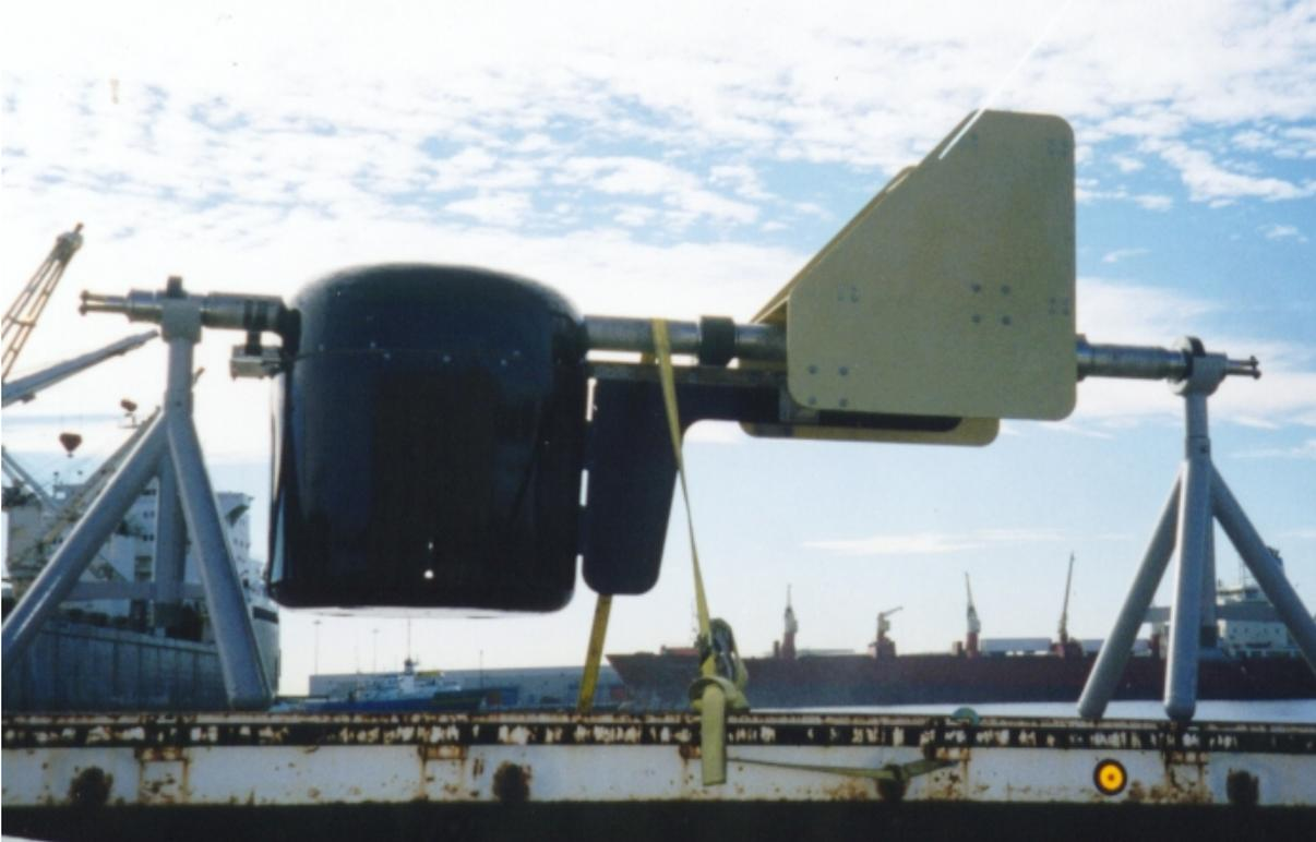
Figure C-4. Photograph of HF/M3 Sonar Towbody on Storage Stands.
