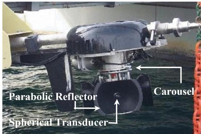
Figure 3. Detailed view of system without lower fairing being deployed at Naval Underwater Warfare Center (NUWC) sonar test facility, Seneca Lake, NY.
