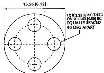
FIGURE 2 Rotator shaft attachment, Acoustic Pressure Tank Facility
