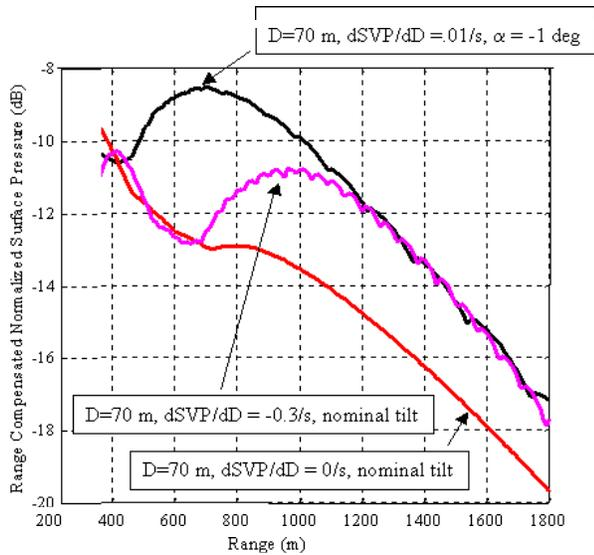
Figure AA - 6 – Predicted normalized surface pressure for various sound velocity and tilt configurations. The highest levels are associated with the configurations studied here. The remaining curves are associated with optimal tilt settings for various sound velocity profile slopes and system depths.
