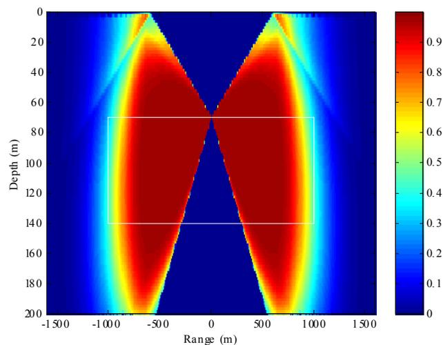
**Figure AA-11. Probability of detecting  $-4$ dB target at various field points for uniform sound velocity.**
