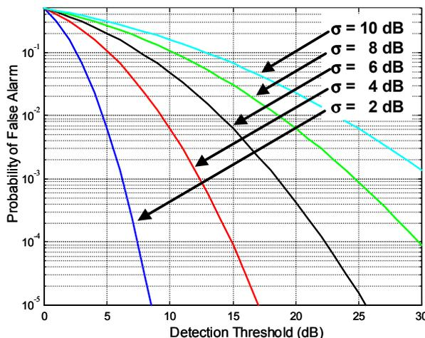
**Figure AA-8. Probability of false alarm for several noise level variances as a function of detection threshold. The noise probability distribution function is assumed to be Gaussian.**
