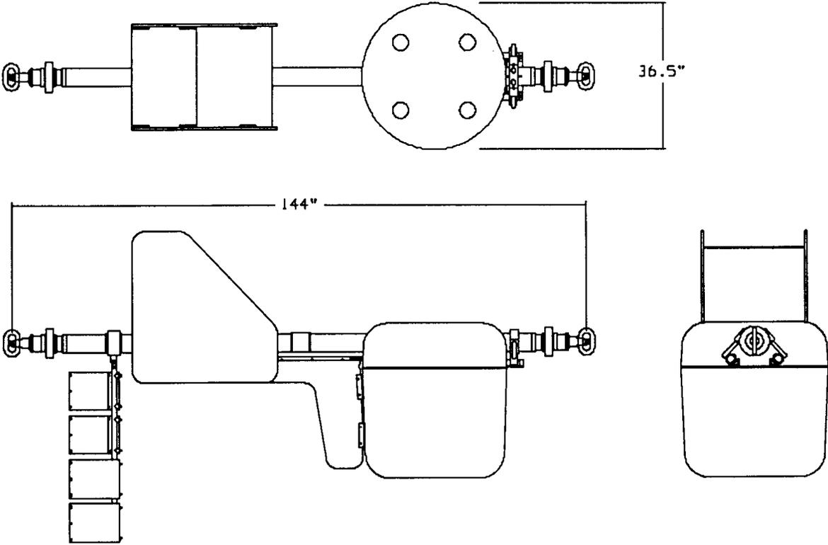
Figure C-2. HF/M3 Sonar Towbody, Orthographic Views.
