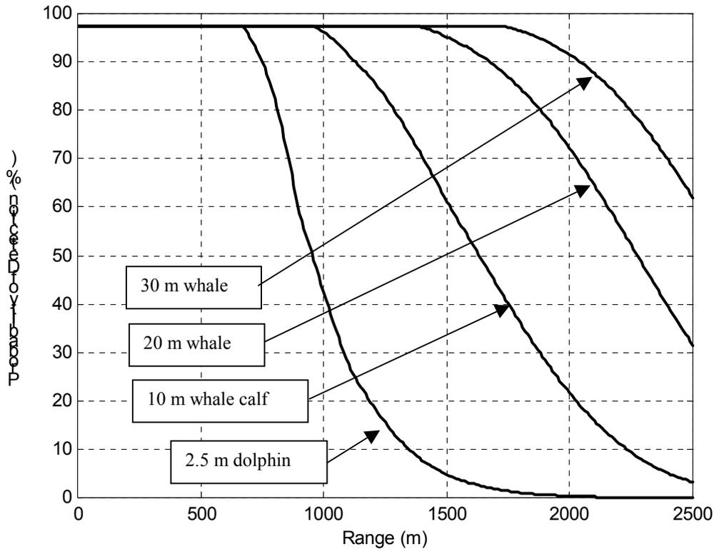
Figure B-22. Probability of Detecting (on any given ping) Various Marine Mammals Swimming within the Search Beam of the HF/M3 Sonar System.
