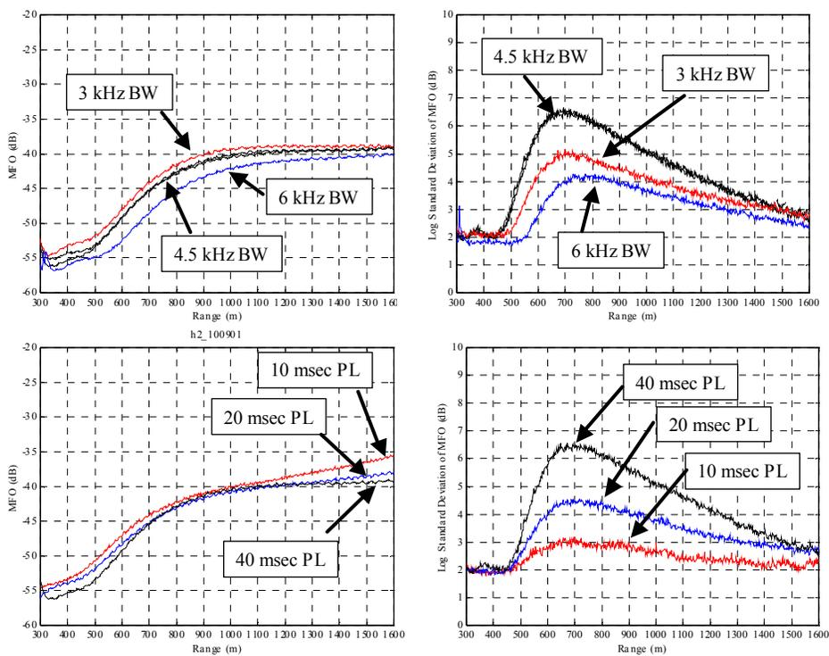
Figure AA-7. Effect of waveform parameters on mean interference level and interference levels standard deviations. The BW variations are performed with a fixed 40 msec pulse length, and the pulse length variations are performed with a fixed 4.5 kHz bandwidth. All cases have a  $-1.5$  degree tilt setting.
