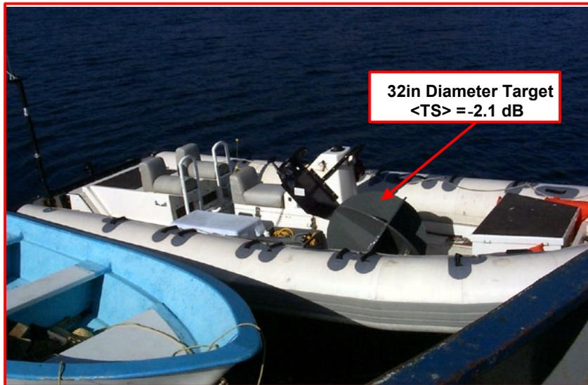
Figure B-8. RHIB with the 32 inch Diameter Target (TS = -2.1 dB).
