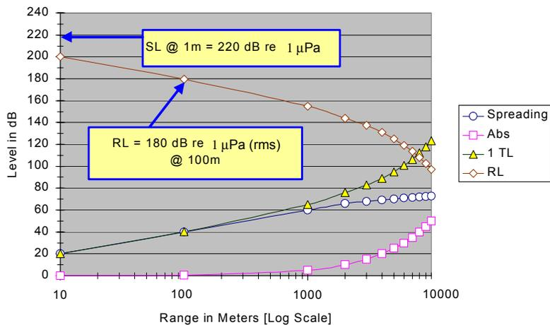
Figure A-4. HF/M3 System One-Way Transmission Loss to 10 km.
