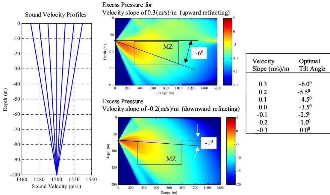
**Figure AA-2. Potential sound velocity profiles, simulated spreading compensated transmission loss for two cases and optimal tilt settings for the various profile slopes and system depth of 70 m.**
