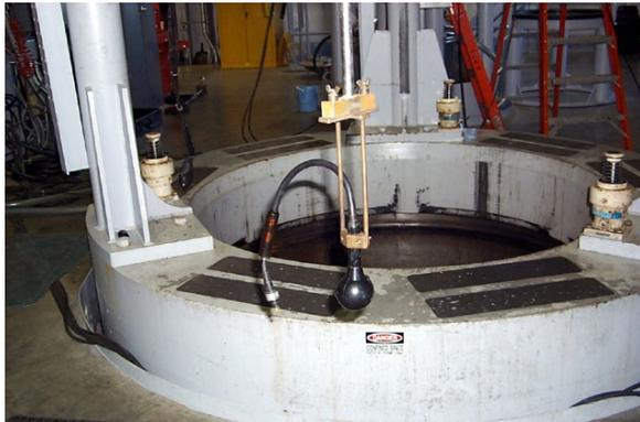
Figure B-13. Bare ITC 1032 Transducer Rigged for Testing in the Acoustic Pressure Tank Facility.
