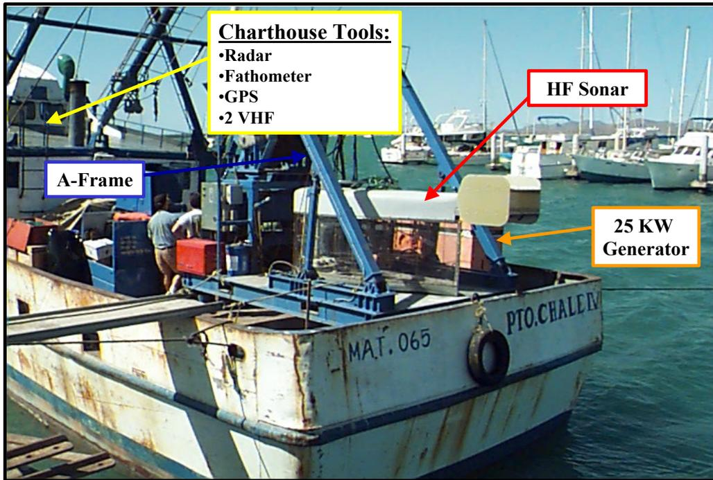
Figure B-4. HF/M3 Test Vessel Showing A-Frame and HF System Fairing Body.
