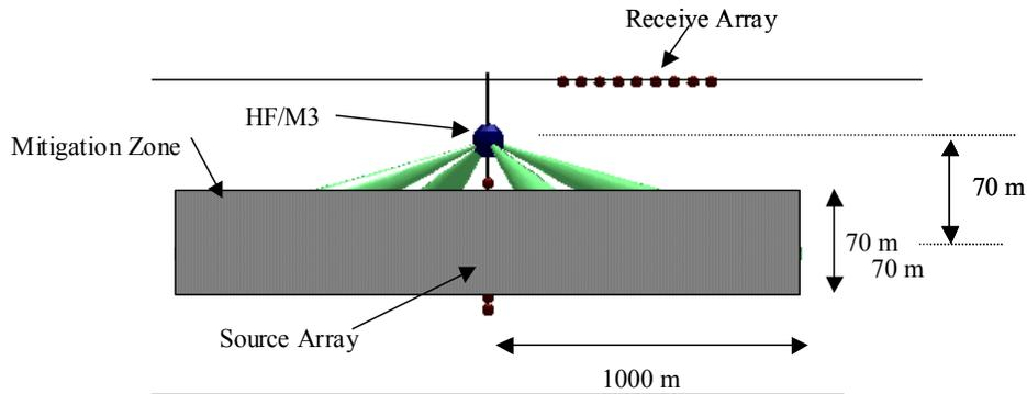
**Figure AA-1. System concept and definition of the LFA Marine Mammal Mitigation Zone (MZ) (figure is not to scale).**
