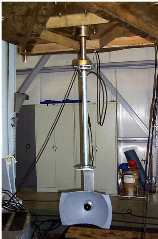
Figure B-14. Parabolic Reflector with an ITC 1032 at the Focal Point, Mounted on the Mechanical Rotator Unit.
