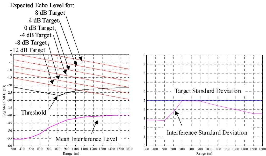
**Figure AA-9. HF/M3 thresholding scheme. The left hand figure shows the mean interference, threshold level and predicted mean echo levels for various target strengths. The right hand figure shows the standard deviation of interference and targets. All probability distribution functions are assumed Gaussian.**
