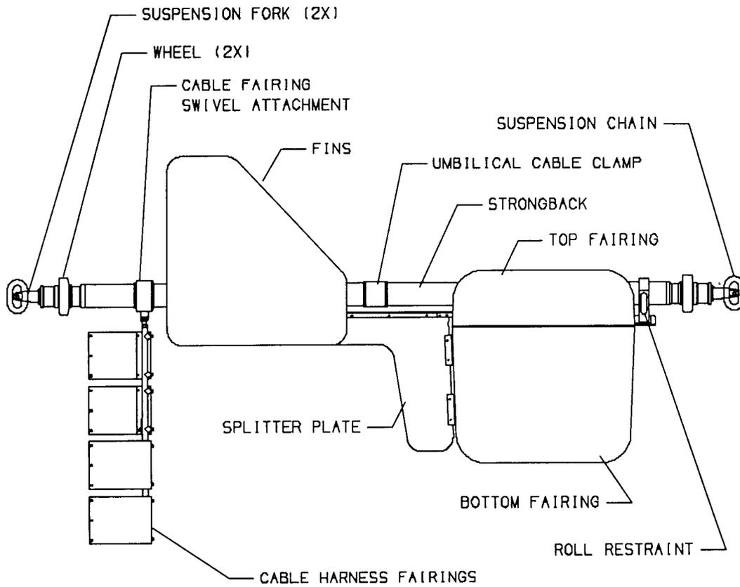
Figure C-3. HF/M3 Sonar Towbody Components.
