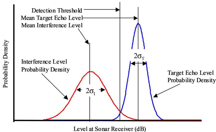
**Figure AA-3. Illustration of target level probability density, interference level probability density and detection threshold.**
