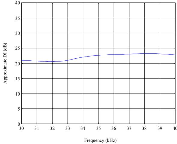
Figure B-17. Approximate Directivity Index (DI) of the Parabolic Reflector, Obtained by Subtracting the Nominal Bare Hydrophone Measured TVR from the Measured On-axis TVR of the Parabola.
