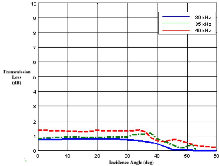
Figure B-20. Fiberglass Transmission Loss Curves versus Incidence Angle for Frequencies 30-40 kHz
