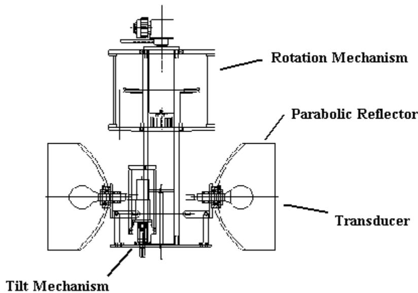
Figure C-6. Omni-directional Transducers Mounted in Parabolic Reflectors.
