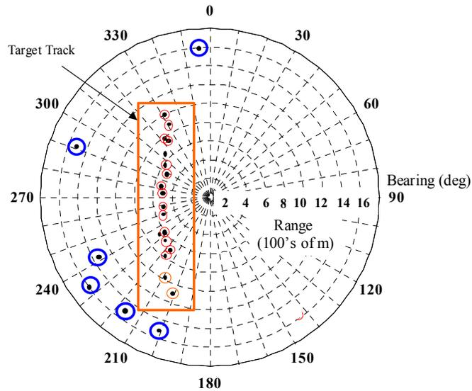
**Figure AA-5. Tracking run detections (tilt of  $-1.3$  deg, BW of 4500 Hz, pulse length of 20 msec). Black dots are instances when the threshold level was exceeded. Detections that are circled in red are associated with a stationary deployed target with TS of  $-8$ dB. Detections circled in blue are considered false alarms. 6 false alarms, the majority occurring beyond 1400 m, occurred during the 30 azimuthal sweeps shown.**
