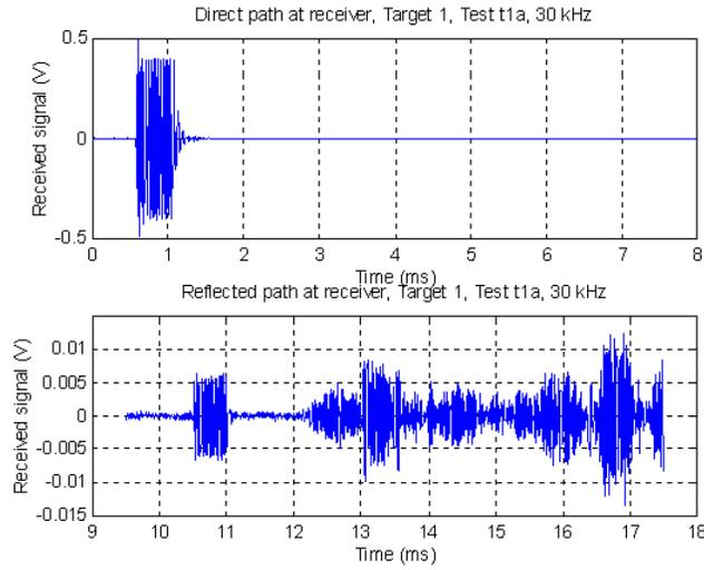
Figure B-3. Typical Signals, Direct Path and Reflected Path
