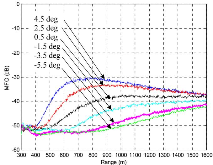
**Figure AA-4. Effect of tilt on mean interference level.**
