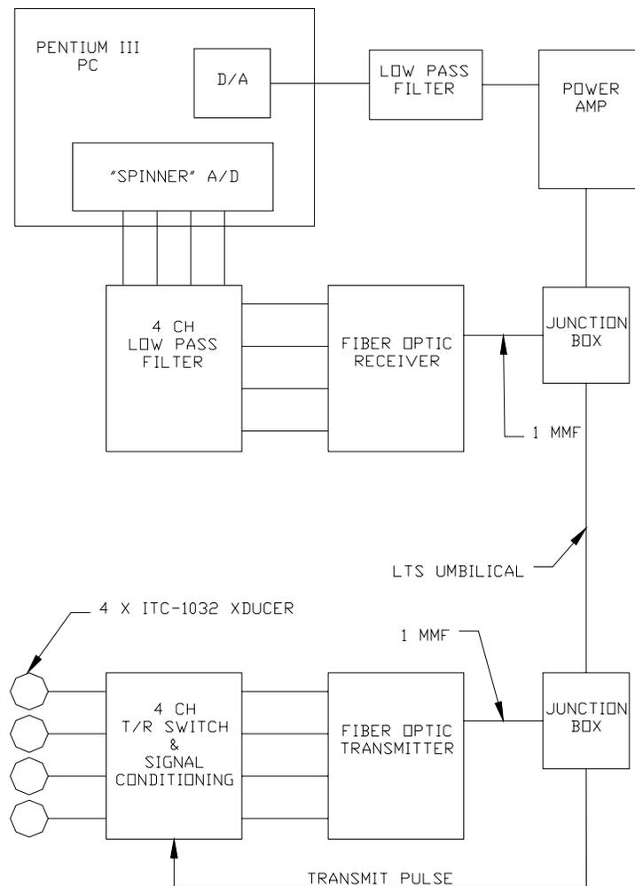
Figure C-1. Key Components of HF/M3 Sonar System.
