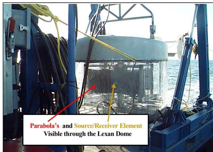
Figure A-5. HF/M3 Sonar Prototype.
