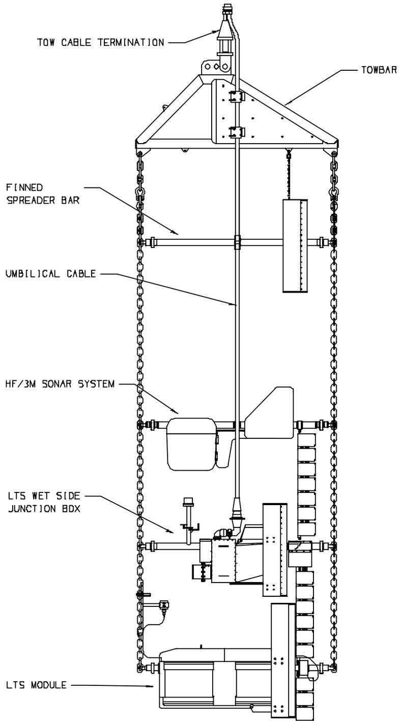
Figure C-5. Top Portion of LTS Array with HF/M3 Sonar System.
