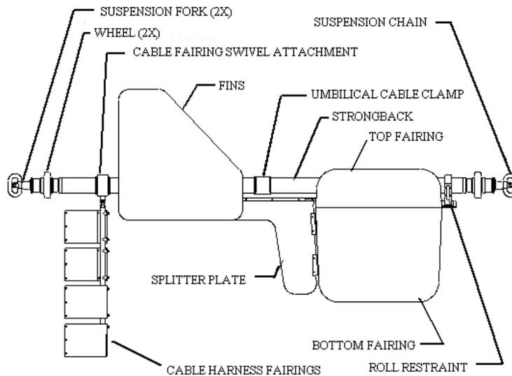
Figure A-7. Schematic of the HF/M3 Sonar Installed on R/V *Cory Chouest*.
