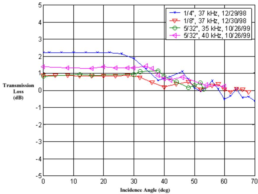
Figure B-21. Transmission Loss Curves for Previous Tests of Fiberglass Panels.
