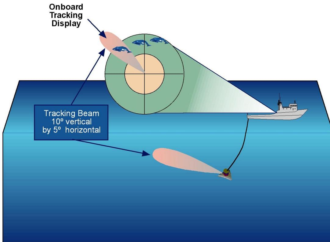
Figure B-6. HF/M3 Sonar Baja Test Configuration.
