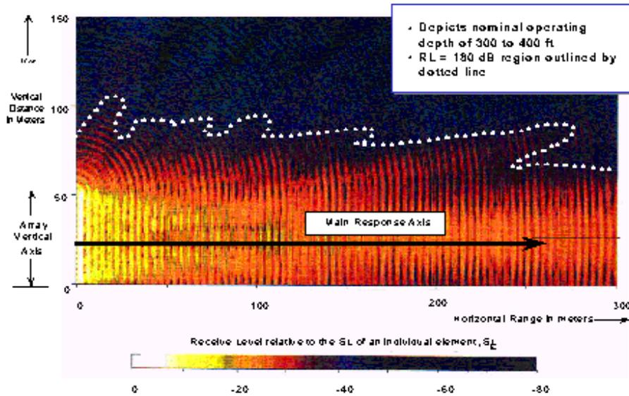
Figure A-2. Transmitted Near Field Sound Levels From a Low Frequency Multi-Element VLA.
